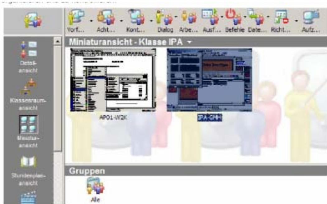
The software consists of two parts, one of that is called “student” running on the PC to be controlled. The other part is called “teacher” and is installed on the Master PC.
